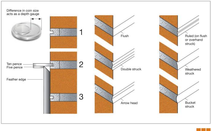
**Bucket handled or Curved Recessed:** This joint gives good weather resistance. The cement is bought to the surface by working the joint for improved weather resistance. The joint is both economical and the most commonly chosen joint. Owing to the compressing of the joint and the superior bond, it has good weather resistance and is suitable for all grades of exposure. It is normally a one operation finish not relying on a follow on pointing operation.
